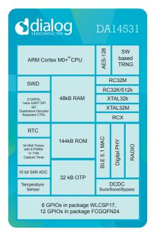
Record low hibernation and active power consumption ensure long operating and shelf life with even the tiniest, disposable batteries. Based on a powerful 32-bit arm Cortex M0+ with integrated memories and a complete set of analog and digital peripherals, SmartBond TINY<sup>TM</sup> is extremely power efficient, delivering a record score of 18300 on the latest EEMBC benchmark for IoT connectivity, IoTMarkTM.
