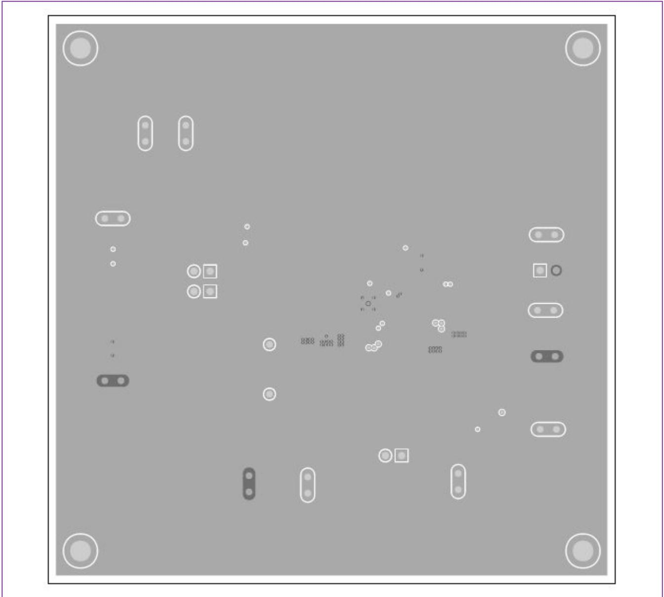
MAX20414 EV Kit Schematic PCB Layout—Internal Layer 2
