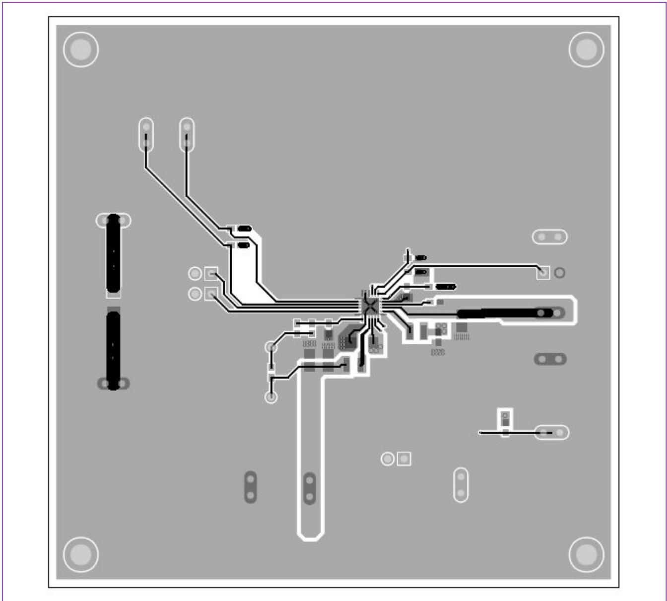
MAX20414 EV Kit Schematic PCB Layout—Top Layer
