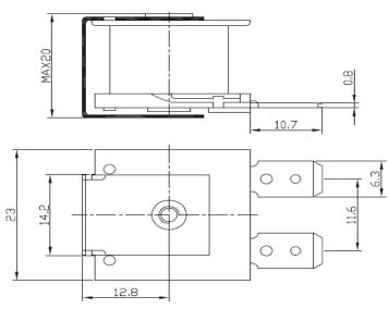
Dimensions : Millimetres Tolerance: ±0.5mm
