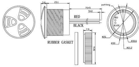
Dimensions : Millimetres Tolerance: ±0.5mm
