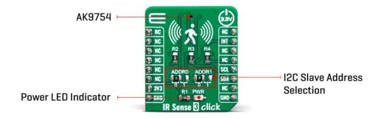
The chip comes with the factory calibrated offset, making the IR Sense 3 click ready to be used out of the box. The sensor data is output through the I2C bus, with its pins routed to the appropriate mikroBUS<sup>™</sup> pins. The I2C interface supports both normal (clock speed up to 100kHz) and fast mode (clock speed up to 400kHz).
