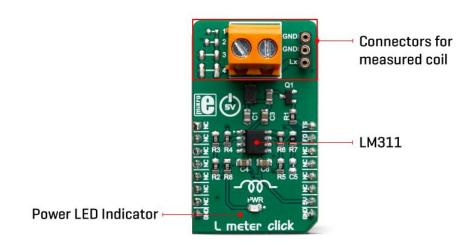
This Click board™ is designed to use only next mikroBUS™ pins: PWM output as a Trigger signal and INT – Hardware Interrupt that receive a square wave frequency output from Click board™. Pins PWM and INT and are labeled as TS and FO, respectively. The board has two type of terminals for a coil connection: TB1 screws terminals and TS2 female header terminals. L meter click also have four blank SMD places, to allow soldering different SMD coils for measuring directly onboard.
