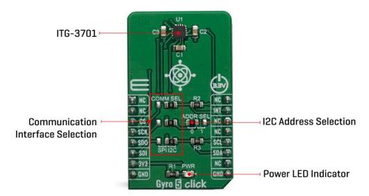
Typically, higher dps range results in lower sensitivity. Therefore, the ITG-3701 allows to dynamically select the full-scale range (FSR) value in several discrete steps: ±500, ±1000, ±2000 and ±2000 dps. This allows optimized performance for a given usage scenario. For example, if used in applications with faster angle rates such as sports equipment monitoring (golf club or tennis racket), a higher FSR might be required, at a cost of lower sensitivity.
