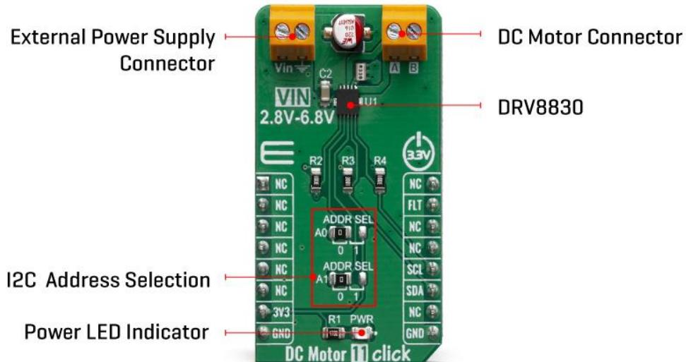
The DRV8830 includes an internal reference voltage that is connected to a DAC. This DAC generates a voltage which is used to set the PWM regulated output voltage, and therefore speed and direction of the motor rotation. The DAC is controlled by the VSET bits from the I2C interface. For the detailed commands for desired output voltages, refer to DRV8830 datasheet.
