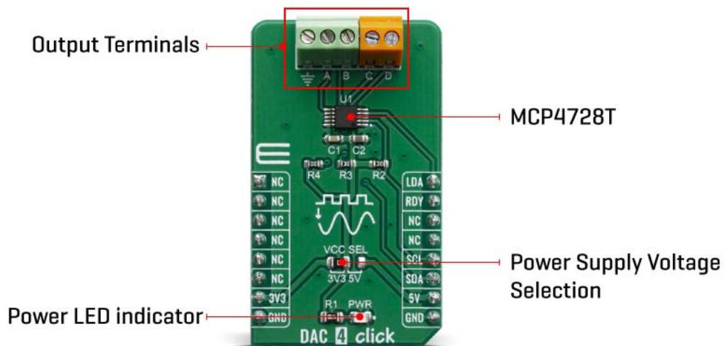
The MCP4728 device has a high precision internal voltage reference ( $V_{REF} = 2.048V$ ). The internal reference can be selected by user, or external reference may be used ( $V_{DD}$ ) for each channel individually. This gives the DAC 4 click good flexibility for use in various applications.
