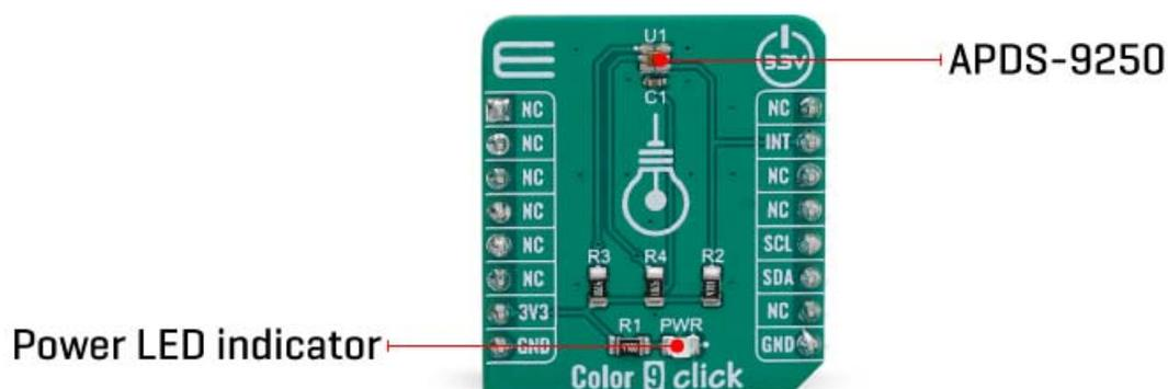
The color intensity sensing is roughly matched to the sensitivity of the human eye, so the sensor is the most sensitive in the range between 500nm and 600nm. The datasheet of the APDS-9250 offers an intensity over the wavelength diagram, so an accurate color calculation can be made in respect to the variable sensitivity of the sensor over the light wavelength.
