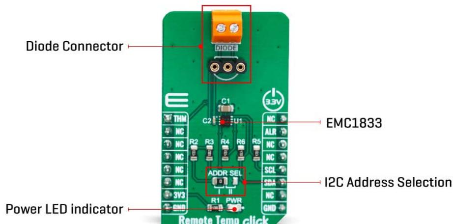
There are some specific requirements for a discrete component when using it as a remote temperature sensor: for example, it has to be a small signal BJT. For more information, please refer to datasheet of the EMC1833, which also states some forward voltage ranges for the highest and the lowest expected temperatures and other parameters which should be considered when selecting the transistor. The discrete component can be connected to the screw terminal at the edge of the Click board™.
