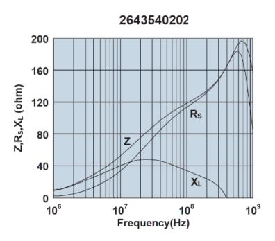
Impedance, reactance, and resistance vs. frequency.
