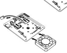
6. Route the wire neatly under the lugs on the fan support and connect the fan wiring to the two pin header on the PCB noting the polarity as shown.
