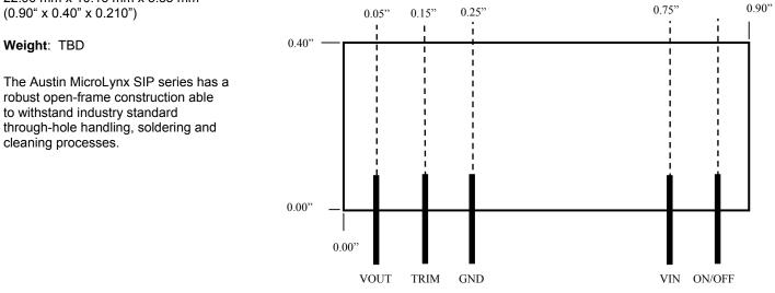
Pin diameter =  $0.51 \text{ mm} (0.02^{\circ})$ Module thickness is  $0.210^{\circ} \pm 0.012^{\circ}$
