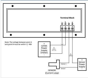
This example illustrates an application where the Current sensor is connected to terminals 3 and 4, where terminal 3 is the negative input terminal (-IN) and terminal 4 is the positive input terminal (+IN).
