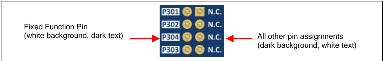
Figure 23. Fixed Function Pin Label Example
