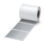
Label for rough surfaces, Roll, silver, unlabeled, can be labeled with: THERMOMARK ROLL 2.0, THERMOMARK ROLL, THERMOMARK ROLL X1, THERMOMARK ROLLMASTER 300/600, THERMOMARK X1.2, mounting type: adhesive, lettering field size: 100 x 90 mm, Number of individual labels: 250
