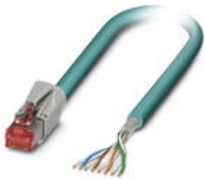
Assembled Ethernet cable, CAT6, shielded, 4-pair, AWG 26 stranded (7-wire), RAL 5021 (water blue), RJ45 plug/IP20 on free conductor end, line, length 2 m
