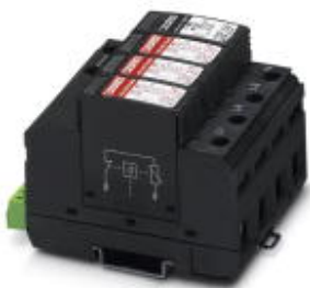
Surge voltage arrester combination 4-channel, for mounting on NS 35/7.5, with remote indicator contact as PDT, voltage 230 V AC
