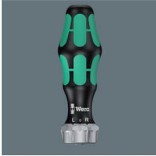
Suitable for 6 mm Wera Vario blades. Ratchet, fine-tooth design for minimal return angle, switchover ring (right, locked, left), maximum torque of up to 50 Newton metres, 6 mm hexagon chuck.
