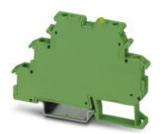
Input solid-state relay terminal block, input: 120 V DC, output: 3 - 48 V DC/100 mA, terminal block width: 6.2 mm
