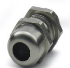
Cable gland, cable gland material: Stainless steel 1.4305, external cable diameter 5 mm ... 10 mm, shielding: no, connecting thread: M16 x 1.5, color: silver, with O-ring
