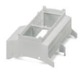
DIN rail housing for use in distribution boards in accordance with DIN 43880, Upper housing part, width: 107.6 mm, height: 89.7 mm, Depth: 54.85 mm, color: light gray (7035)
