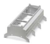
DIN rail housing for use in distribution boards in accordance with DIN 43880, Upper housing part with vents, Installation depth connection technology: 11.1 mm, width: 161.6 mm, height: 89.7 mm, Depth: 54.85 mm, color: light gray (7035)
