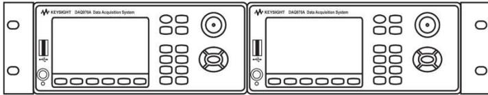
To rack mount two instrument side-by-side, order the lock-link kit (part number: DAQ194A) and flange kit (part number: DAQ191A)
