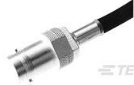
TE Model / Part #1- 1337441-0 BNC Str Jk Hex 50Ohm Nickel Pltd RG58C/U
