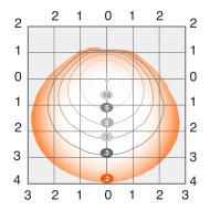
SLMFLD1A/100UNV8X0/WF/BZ Isofootcandle Lines at 10' Mounting Height
