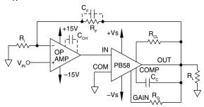
Figure 2. Non-inverting composite amplifier.
