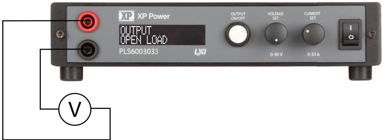
When the volt meter is connected, press the output on/off button. The following screen is an example of what will appear.
