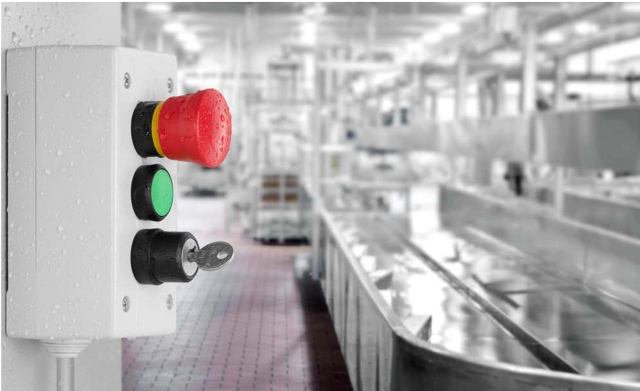
Machines covered by the Machinery Directive (2006/42/EC) must be equipped with at least one emergency stop actuator that can prevent an imminent or occurring hazard.
