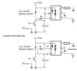
To ensure that the product operates correctly, use the following formula to calculate the limiting resistance, and design the circuit accordingly.
