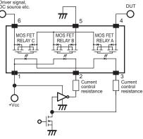
Note: The number from 1 to 6 are the pin numbers in the image shown here.
