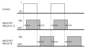
\* This products is recommended to use with dry switching (No Load & No Source when switching) for prevent short circuit happening.
