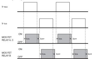
\* Both MOS FET relay A, C and MOS FET relay B may be ON at the same time. For that reason, even if pins 4, 5 and 6 are all connected, please design the circuit so that the equipment does not occur the damage.
