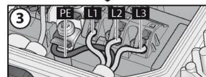
Fig. 3: Connecting the wires to terminals
