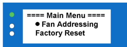
Figure 5 - Main menu display screen on first application of power
