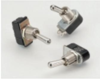
The 110-Series is a compactly designed, versatile metal construction toggle switch. Features include single or double pole options, maintained or momentary construction with termination choices including solder lug end or bottom, wire leads and .250 tab terminals. The quick make/quick break contact mechanism makes the switch suitable for high voltage (125-250 volt) applications. This switch is popular within the Small Appliance, Floor Maintenance, and most low current AC/DC market segments.
