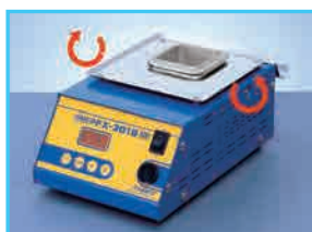
Loosen the screw on both sides.
