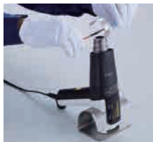
Heat shrink tubing Use of hook type nozzle and stand
