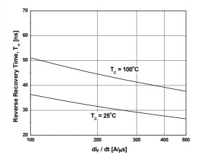
Figure 7. Typical Reverse Recovery Current
