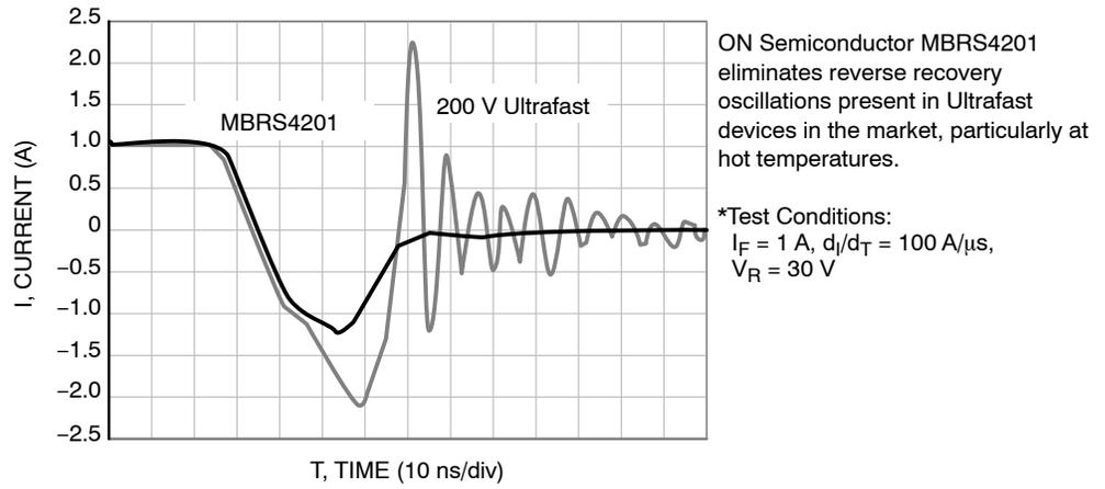
Figure 8. Reverse Recovery Time\* ( $t_{RR}$ ) at 125°C
