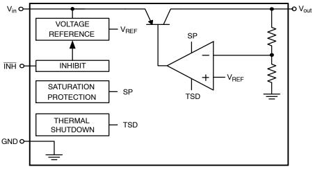
Figure 2. Simplified Block Diagram
