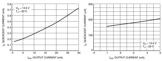
Figure 8. Quiescent Current vs. Output Current (High Load)
