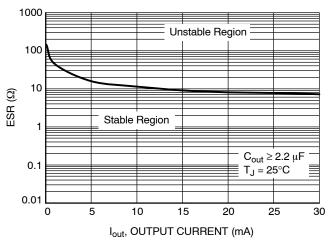
Figure 11. Output Stability with Output **Capacitor ESR**
