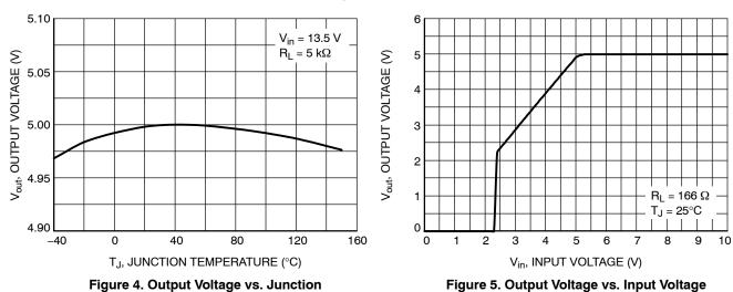
Figure 4. Output Voltage vs. Junction **Temperature**
