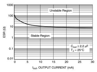
Figure 3. Output Stability with Output **Capacitor ESR**
