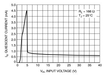
Figure 10. Quiescent Current vs. Input Voltage
