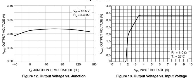
Figure 12. Output Voltage vs. Junction **Temperature**
