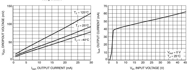
Figure 6. Dropout Voltage vs. Output Current
