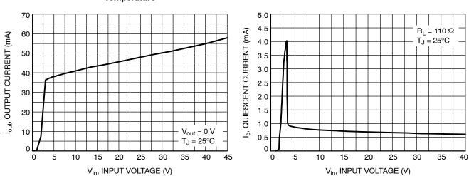
Figure 14. Maximum Output Current vs. Input Voltage
