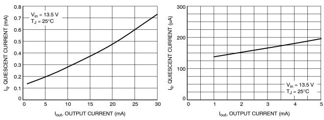
Figure 16. Quiescent Current vs. Output Current (High Load)
