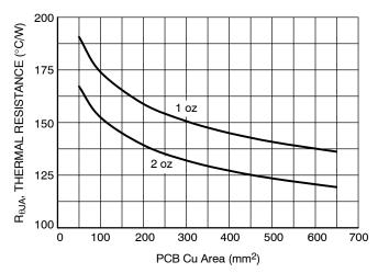
Figure 18.  $R_{\theta JA}$  vs. PCB Cu Area
