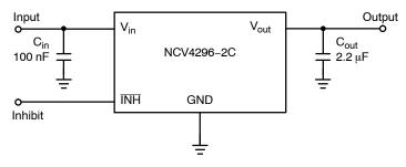
Figure 1. Applications Circuit
