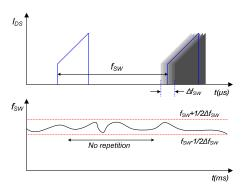
Figure 27. Random Frequency Fluctuation
