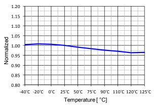
Figure 15. Switching Frequency (fs) vs. TA
