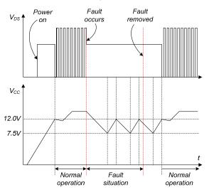
Figure 21. Auto-Restart Protection Waveforms
