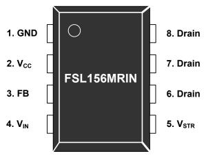
Figure 3. Pin Assignments (Top View)
