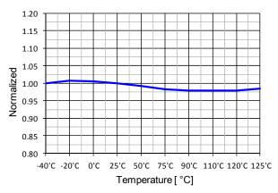
Figure 5. Operating Supply Current (IOP) vs. TA
