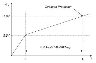
Figure 22. Overload Protection
