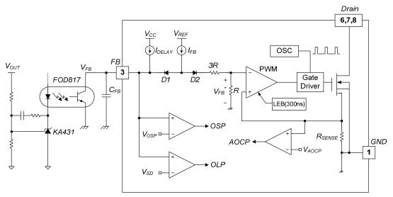
Figure 20. Pulse Width Modulation Circuit
