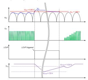
Figure 25. Line Over-Voltage Protection
