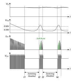
Figure 26. Burst-Mode Operation
