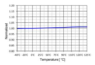
Figure 12. UVLO Threshold Voltage (V<sub>STOP</sub>) vs. T<sub>A</sub>
