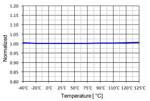
Figure 13. Shutdown Feedback Voltage (V<sub>SD</sub>) vs. T<sub>A</sub>
