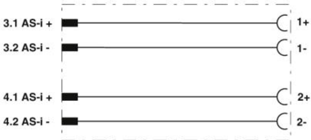
Contact assignment of the AS-Interface distributor
