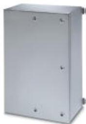
Junction box, material: Stainless steel, 316L/1.4404, surface resistance: brushed, silver, 600 mm x 800 mm x 300 mm, type of locking: Door with replaceable hinge, scope of supply - ATD: Door hinge with quarter turn locking, Mounting plate, Double-bit key, Fixing angle with mounting screws, M12 grounding bolts, affixed externally, Installation notes, Door hinge with quarter turn locking
