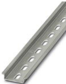
DIN rail perforated, Standard profile, width: 35 mm, height: 7.5 mm, acc. to EN 60715, material: Steel, uncoated, length: 2000 mm, color: white aluminum
