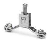
Ground modular terminal block, connection method: Screw connection, number of connections: 2, number of positions: 1, cross section: 0.5 mm² - 16 mm², AWG: 20 - 6, width: 8 mm, color: silver, mounting type: NS 35/7,5, NS 35/15
