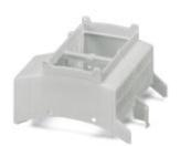
DIN rail housing for use in distribution boards in accordance with DIN 43880, Upper housing part with vents, width: 71.6 mm, height: 89.7 mm, depth: 54.85 mm, color: light gray (7035)
