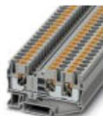
Feed-through terminal block, nom. voltage: 1000 V, nominal current: 41 A, connection method: Push-in connection, number of connections: 3, cross section: 0.5 mm<sup>2</sup> - 10 mm<sup>2</sup>, AWG: 20 - 8, width: 8.2 mm, height: 42.2 mm, color: gray, mounting type: NS 35/7,5, NS 35/15
