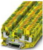
Ground modular terminal block, connection method: Push-in connection, number of connections: 3, cross section: 0.5 mm<sup>2</sup> - 10 mm<sup>2</sup>, AWG: 20 - 8, width: 8.2 mm, height: 42.2 mm, color: green-yellow, mounting type: NS 35/7,5, NS 35/15
