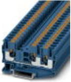
Feed-through terminal block, nom. voltage: 1000 V, nominal current: 41 A, connection method: Push-in connection, number of connections: 3, cross section: 0.5 mm<sup>2</sup> - 10 mm<sup>2</sup>, AWG: 20 - 8, width: 8.2 mm, height: 42.2 mm, color: blue, mounting type: NS 35/7,5, NS 35/15
