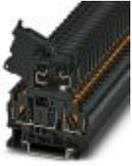
Fuse modular terminal block, fuse type: Glass / ceramics / ..., connection method: Push-in connection, cross section: 0.2 mm<sup>2</sup>- 6 mm<sup>2</sup>, AWG: 24 - 10, nominal current: 6.3 A, nom. voltage: 500 V, width: 6.2 mm, fuse type: G / 5 x 20, mounting type: NS 35/7,5, NS 35/15, color: black
