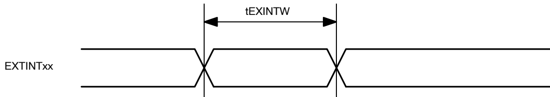
Figure 8. AC Characteristic – External Interrupt
