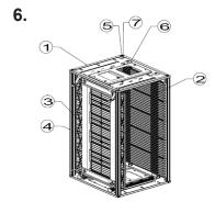
Fasten the screws on fixed side board and pull several times of the movable side board, to see whether synchro or out of gear, installation finished (picture above).
