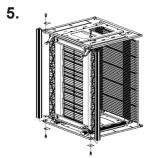
Install four aluminium-alloy stanchions, Pad gasket, Fasten the screws (picture above)
