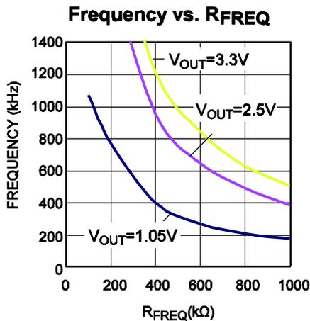
Generally, the NB638 is set for 200 kHz to 1MHz application. It is optimized to operate at high switching frequency with high efficiency. High switching frequency makes it possible to utilize small sized LC filter components to save system PCB space.
