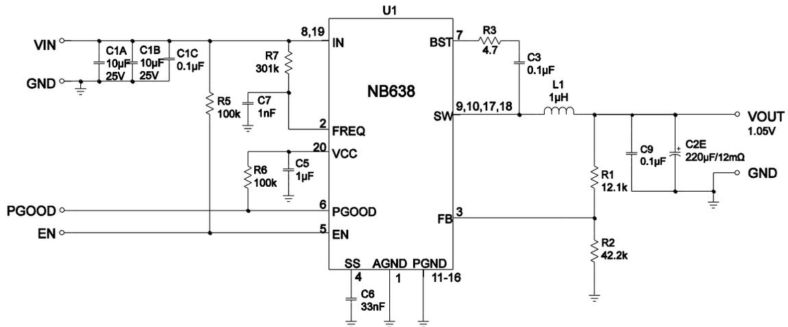
**Figure 12 — Typical Application Circuit with No External Ramp**
