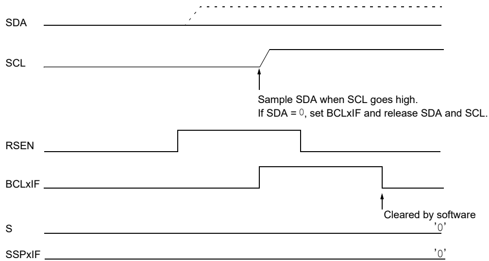
Figure 29-36. Bus Collision During a Repeated Start Condition (Case 1)
