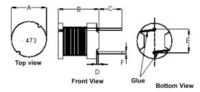
Note : White dot of marking indicates the start terminal of winding
